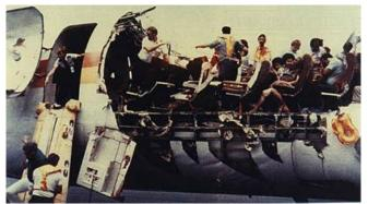
Aloha Airlines, Flight 243, April 28, 1988 became known around the world as "the convertible" when it lost 18 feet of the upper fuselage at 24,000 feet. Only one person out of the 95 on board lost her life but the world demanded to know how this could happen to a modern jet transport. This was not the first Boeing 737 to have this type of
